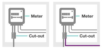
Please note we cannot make joints or extend a cable inside or under the footprint of a building.
