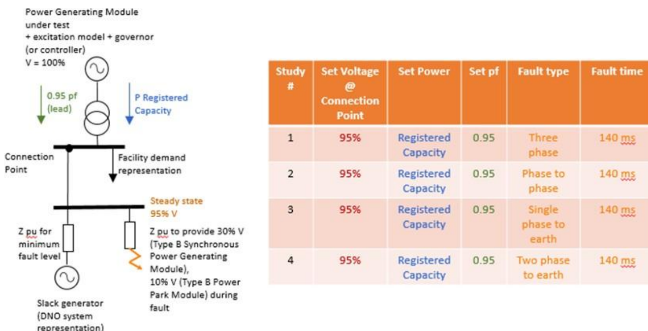
Figure 14: Example of Type B PGM Fault Ride Through and Fast Fault Current Injection Studies.
